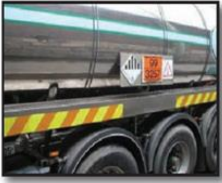
Figure.5.29. Placarding of tanks [45].
